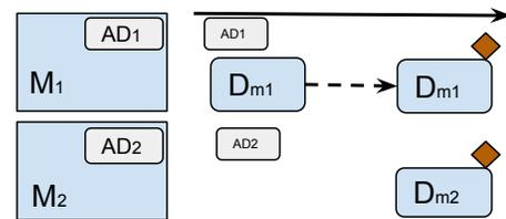
**Figure 2:** Activity Detection Driven (AD): IUs from each modality's ADs signal that data (i.e., IUs) will be forthcoming.  $M_1$  waits for IUs from other  $M_2$  before being passed along. The dashed arrow denotes the IU was received, but held. The solid arrow indicates time.
