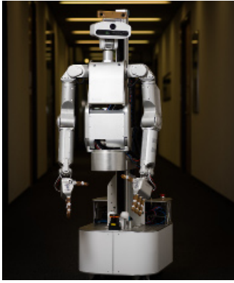
Figure 1. The Meka M1 Mobile Manipulator robotic-platform. Image ©Johannes Wienke
